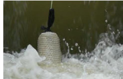
**FLOC ROLL – Polyacrylamide Sediment Removal Roll**
